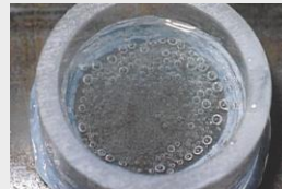
Hydrogen diffusion evident in liquid
