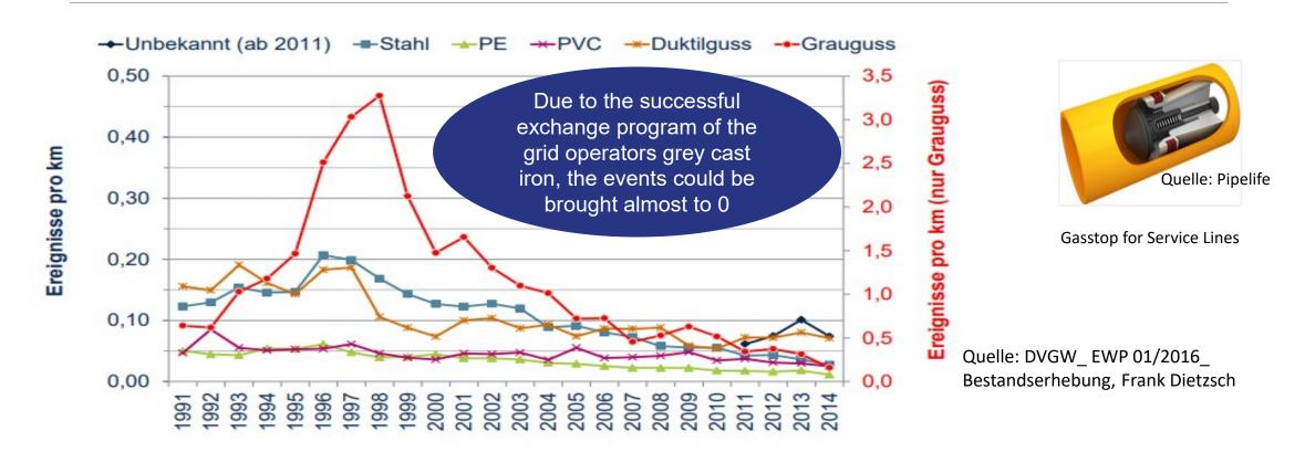
The events per km in German gas distribution networks are already very low; by further expansion of PE networks, the annual events will be reduced even further. In the event of damage by third parties, the amounts of gas released in the HAL area are already limited by a GS. After the grey cast iron exchange program, the network operators are not seeking any further large-scale material exchange.
