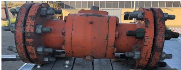
MAPEGAZ (DN150, PN100) valve. Upper stem damaged gasket.
