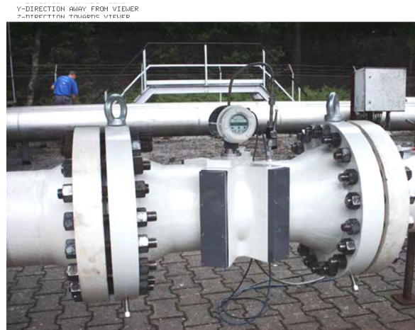
PTB double bend out of plane D=200 mm; Rk=1,5 D 588.6 m 3 /h, 1.005 bar, Re=65000 Turbulence model: RNG k \ \epsilon
