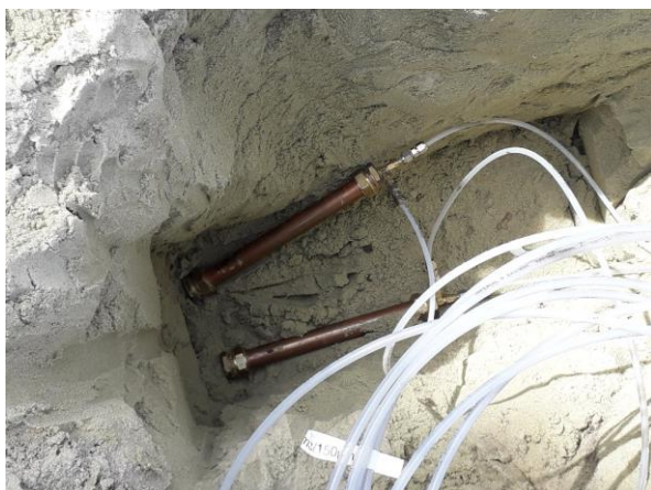
Figure 8 Positioning the leaking pipes in the soil (only a single one at a time was used).
