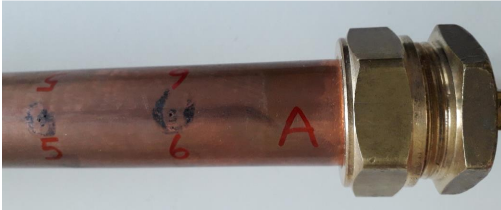
Figure 5 Detail of the pipe and a leak.
