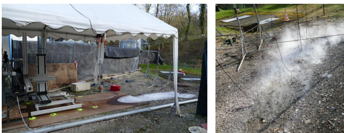
Fig. 11. Test 15 - Pictures showing the rain-out marks after the end of the release
