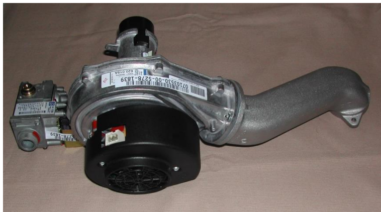
Figure 12: Unit for modern condensing boilers: Fan (motor in black in the front, casing and outlet to the right) venturi (on the back) and gas valve (on the right).
