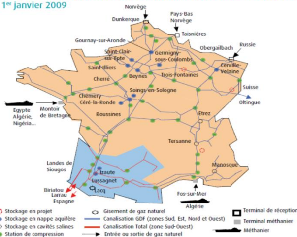
Figure 5: The transport grid, storages, compressor sites and production of natural gas in France (1.1.2009)
